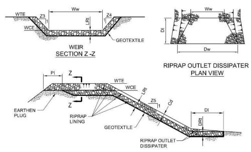
EMBANKMENT SECTION ALONG EMERGENCY SPILLWAY
